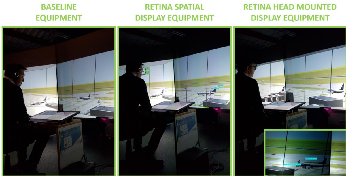
Figure 3 RETINA Validation Platform. The AR App derives the relevant Augmented Reality Overlays and deploys them on the appropriate ATCO Head-Up Interface (being either Spatial Display or Head Mounted Display). The baseline equipment serves to compare data obtained vs success criteria and validation targets identified below.
