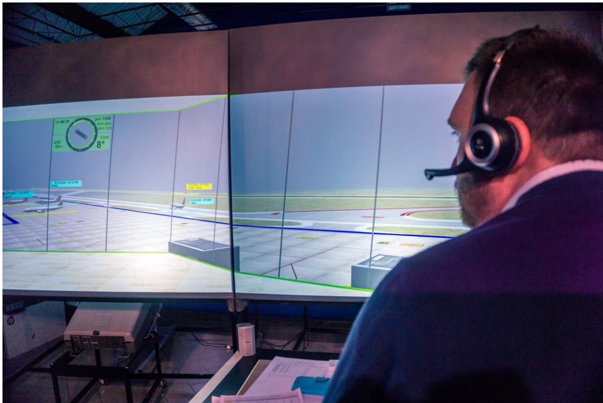
Figure 283 Aircraft labels are displayed near those aircraft/vehicles which fall inside the spatial display range of augmentation
